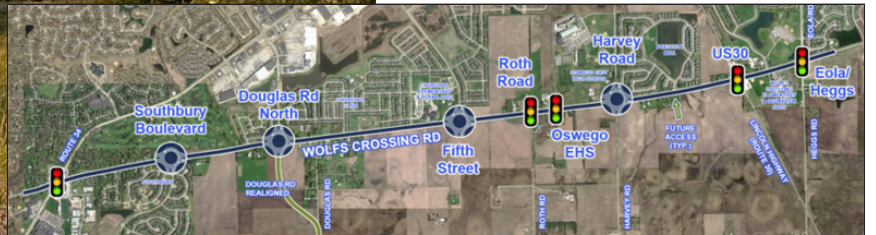
Plans for Wolf's Crossing include additional lanes, stoplight-controlled intersections, realigning Douglas Road, and roundabouts, all of which will improve both safety and traffic flow.
