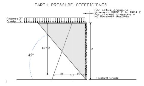
The following table provides the recommended "at-rest" lateral earth pressure coefficients for the soils encountered. Also included are the "active" and "passive" lateral earth pressure coefficients if needed.
