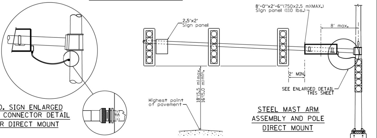
STEEL MAST ARM ASSEMBLY AND POLE DIRECT MOUNT
