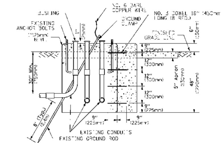
**MODIFY EXISTING TYPE "D" FOUNDATION TO TYPE "C" FOUNDATION**
