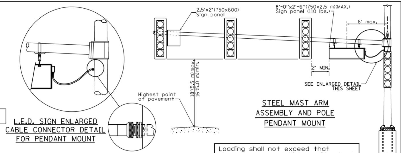
STEEL MAST ARM ASSEMBLY AND POLE PENDANT MOUNT
