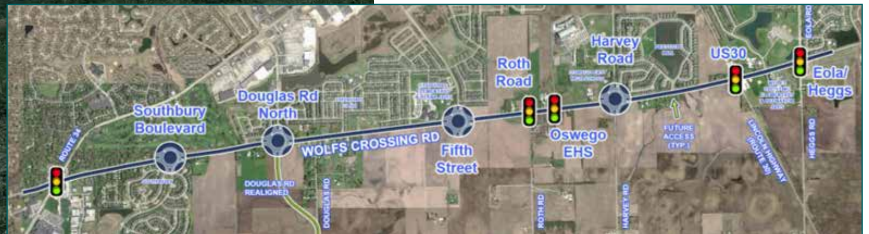
Plans for Wolf's Crossing include additional lanes, stoplight-controlled intersections, realigning Douglas Road, and roundabouts, all of which will improve both safety and traffic flow.
