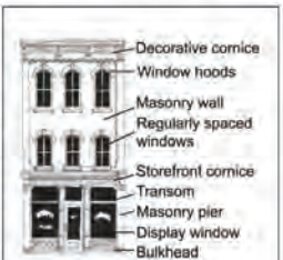
Figure 6.7.5.3: Shopfront Details. This diagram depicts some of the basic architectural components on the primary facade of a Shopfront building.
