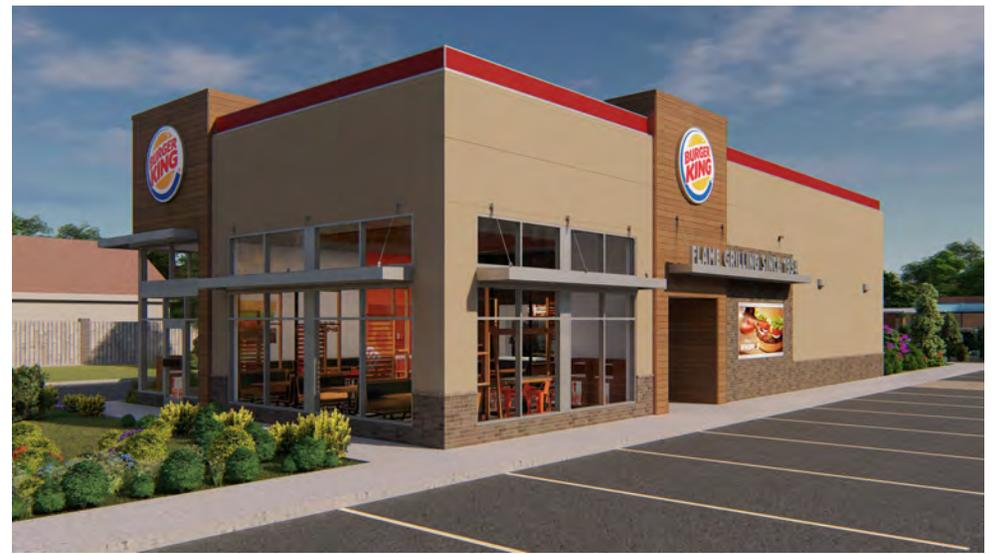
The exterior material is a combination of "Nichiha" cement panels, simulated brick and smooth panels, and EFIS.
