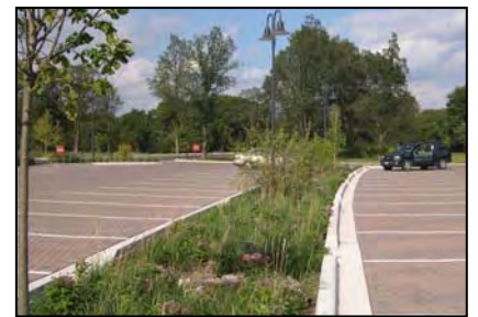
Utilize permeable pavement and water infiltration islands in parking lots
